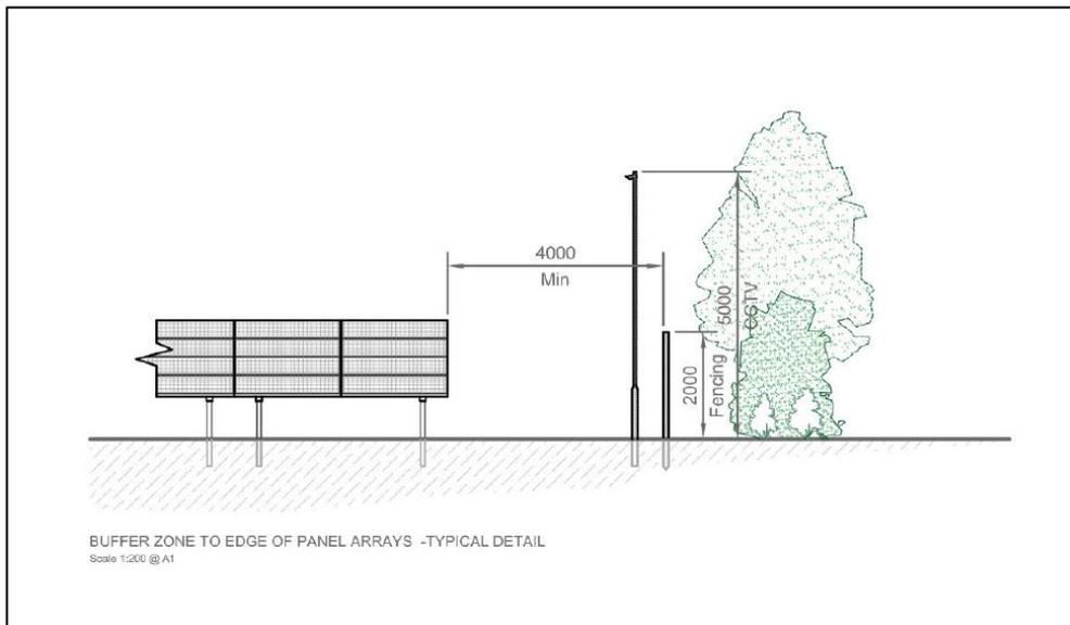
The solar panels will be spaced to avoid shadow and set on a frame supported by stakes. There will be minimal disturbance to the ground, the units also sited to achieve optimum exposure for solar energy absorption. This construction method allows the scheme to be easily reversed in the future, simply by pulling out the framework. There would be no foundations used.
